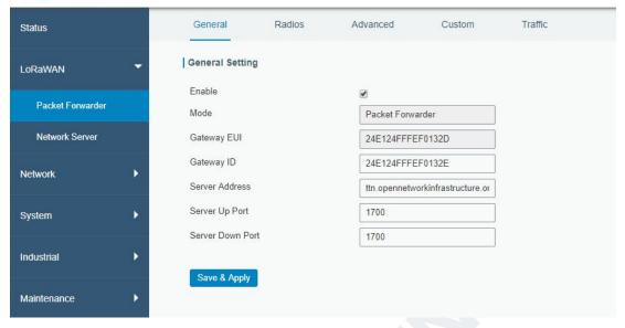
3. Click "Radios" to configure the center frequency and channels.
