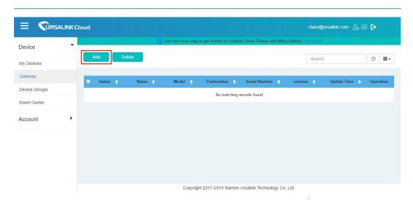
Enter the correct SN of the gateway and click "Add". You can find your gateway SN either on the label on the bottom of the device or on the web GUI.
